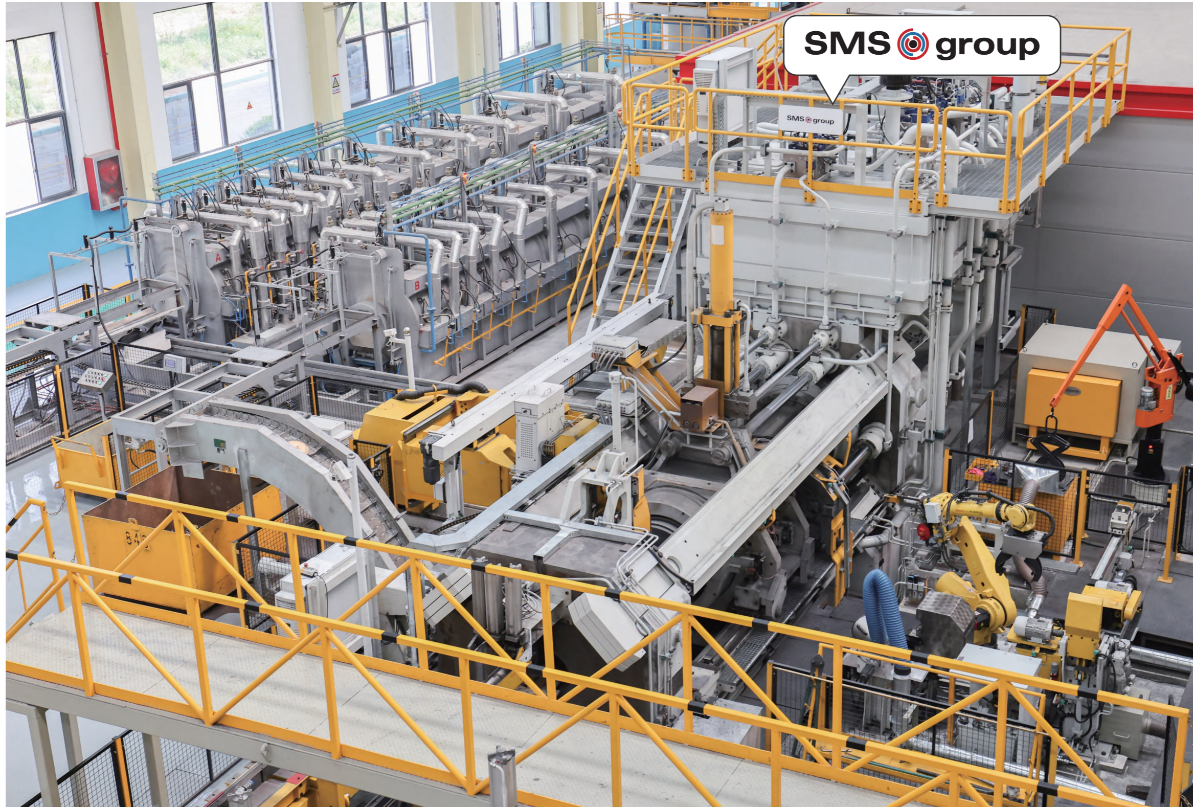
西马克铜及铜合金2800吨反向挤压生产线 28MN Indirect Extrusion Press Line for Copper and Copper Alloys
